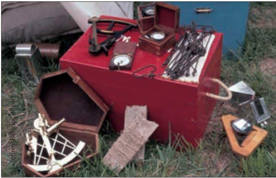
Above are some of the tools used to navigate unknown lands, including a sextant, octant, compass, chronometer, surveyor's chain and artificial horizon.
